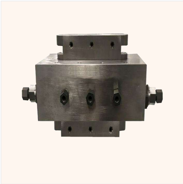
Conductivity cell — front view
