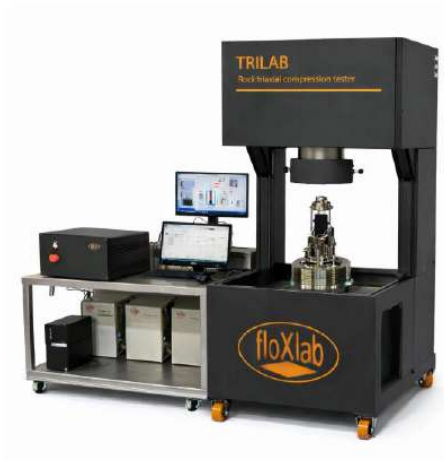
TRILAB — Pressure-balanced triaxial cell with integrated control & acquisition station
