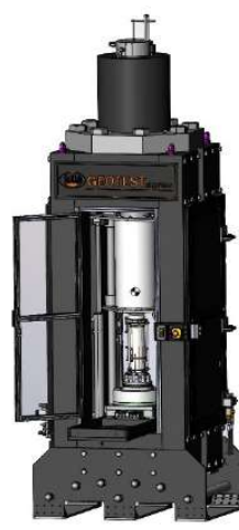
Cell Base Inserted into Load Frame
