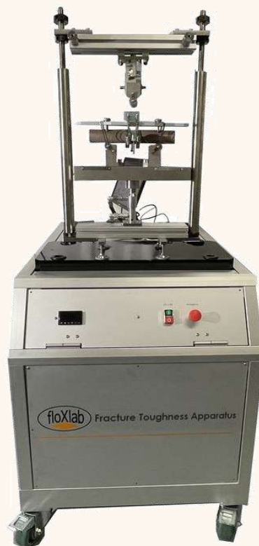
FTA — 10 kN servo-controlled press, ISRM Level I & II compliant
