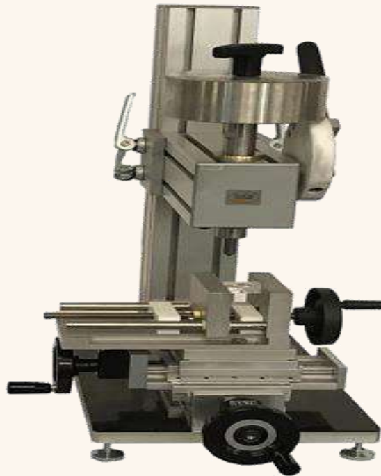
West Cerchar apparatus — fully mechanical hard-rock abrasivity tester
