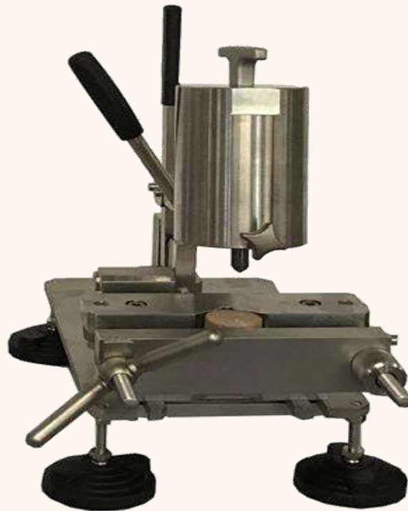
Cerchar Original — fully mechanical hard-rock abrasivity tester
