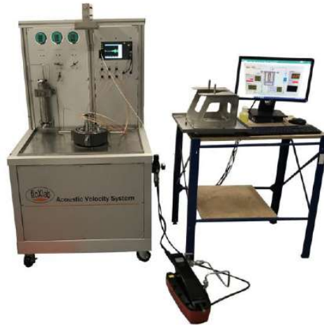
AVS 700 — Standalone acoustic & petrophysical bench for saturated core samples
