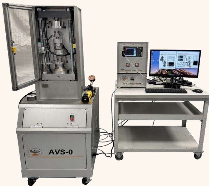
AVS-0 — 300 kN compression frame coupled to acoustic triaxial cell
