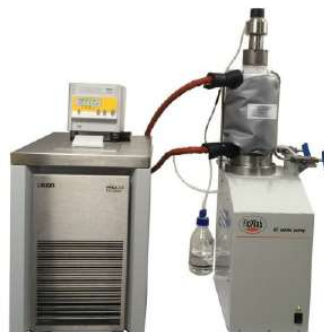
BTSP CO 2 pump with cooling bath
