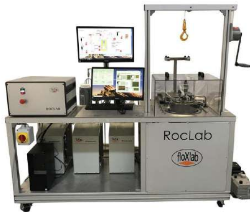
ROCLAB — Automated reservoir-condition compressibility test bench
